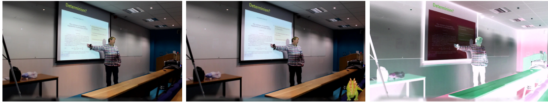
(a) Original video frame (b) Visually watermarked video frame (c) Inverted video frame
